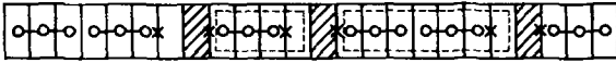
FIG. 7. In this figure, q=6 , N=24 , n_{01}=6 and both end compartments are occupied. There are [n_{01}/2]-1=2 permutable "units" enclosed by a dashed-line box and N-\lambda q-1-[n_{01}/2]-1=3 permutable vacancies (cross hatched). The "units" at each end of the array are not permutable because the compartments at the ends of the array must be occupied.
